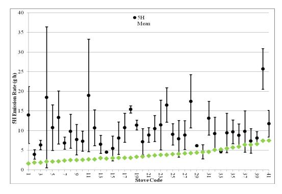
Figure 3. Mean Emission Rates, Standard Deviations around Means, and EPA Certification Values by Heater Model. (Each stove model was assigned a stove code. Green "diamond" symbol is the respective certification value for each stove model.)
